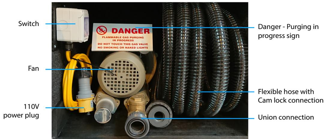
**WARNING:** Do NOT use the unit inside a Hazardous Area, or a in a meter room unless it has been tested and proven to be free of gas. The direct gas to air purge operation is detailed in IGEM UP/1 and UP/1A.
