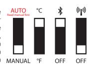
Switches can be adjusted while batteries are removed as well, but note that if you remove the batteries, the measurement history will be erased from Aranet4 memory. The changed preference setting will be enabled once the batteries are inserted back in.
