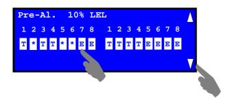
To set other probes, use the **RIGHT** and **LEF**T buttons to move to **probe 7** (in this case) **("E")**. On the first line you will see the gas percentage of "10% LEL".
