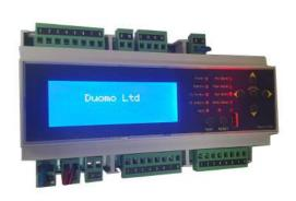
The control unit **BX316/xp** has been designed and built to meet the current requirements of the Market and in compliance with European Standard for checking gas presence in a versatile and innovative using **conventional sensors** Up to 16 remote sensors from 4 to 20 mA can be connected in **conventional** mode for a single area or divided into two zones: 8 sensors for every zone.
