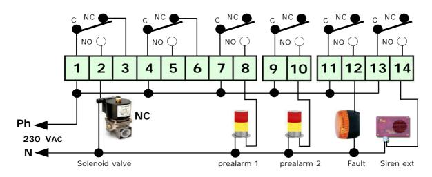
Connecting a Solenoid valve with sirens to 12 VDC, via a power switcing. The power supply should be adequate to the consumption of the components
